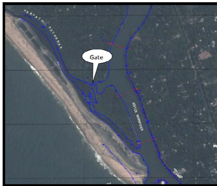
Fig: (6.1) provision of cross regulator at Parvathy Puthanar
