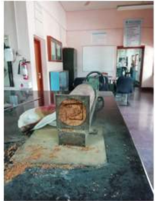
Fig.5 Undisturbed Sample Extracted from core cutter
